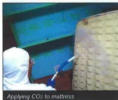
Applying CO 2 to mattress.
